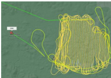
Ignition of Clear Hills, Walpole Wilderness (FRK_086) 9344 ha prescribed burn on 14 October 2023. Incendiaries were dropped 100 m apart on gridlines with 200 m separation. Source: Flight Radar 24.
